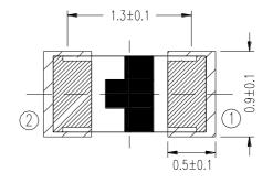
Suggested pad dimension is just for reference only. Please modify the pad dimension based on individual need. Note: Tolerances unless mentioned  $\pm 0.1$ mm. Unit = mm
